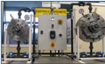
Sealing control test bench
