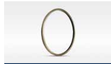
C-FLEX™ METAL SEALS Based on the elastic deformation of a metal "C" substrate which, during the compression cycle, gives a contact point on each sealing surface.
