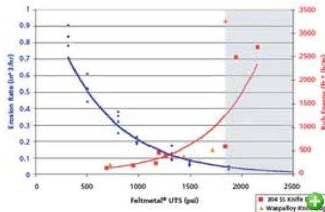
Figure 1. Erosion Rate and Rub Energy vs. Ultimate Tensile Strength
