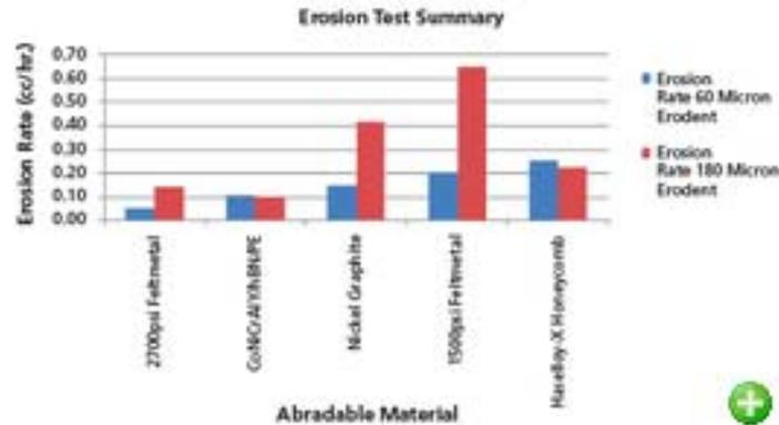
Figure 2. Performance of Various Materials in Erosion Tests
