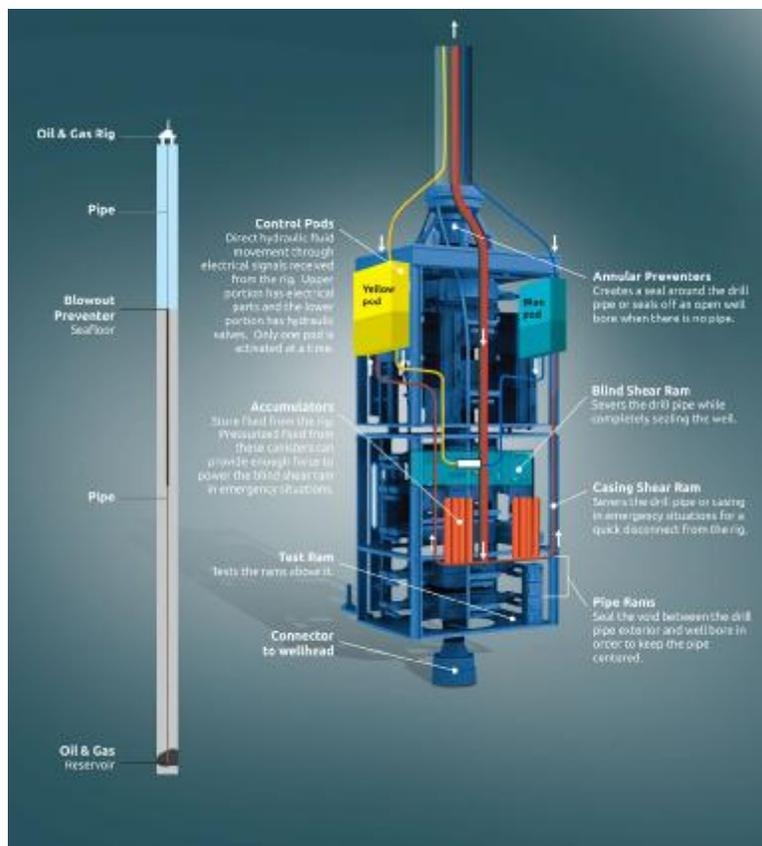
Accumulators are energy storage devices that have a variety of applications. Most notably, they can be used to store potential energy, accommodate fluid expansion or provide damping for pressure transients. Accumulators are typically positioned on the high-pressure side of a system, whereas similar devices on the low-pressure side are referred to as reservoirs. For this discussion, the term accumulator refers to both device types.
