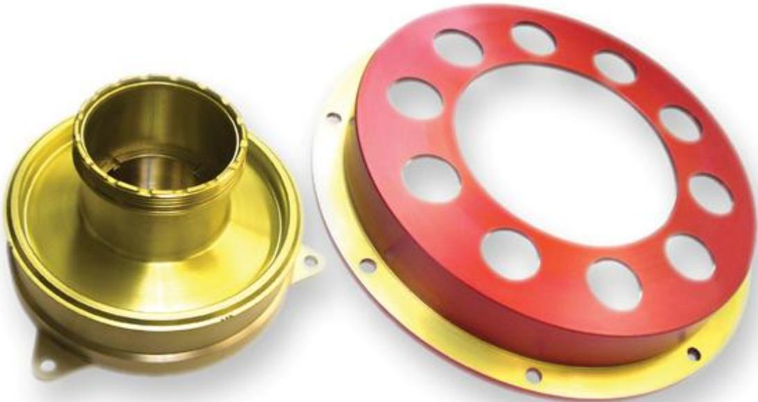
**These low-pressure burst discs are for fueling systems in aircraft. They both protect against pressure surges and are compatible with jet fuel. Burst discs for aerospace applications are made of aluminum, stainless steel, superalloys, PTFE, and other materials compatible with jet and rocket fuels, oxidizers, and other harsh fluids.**
