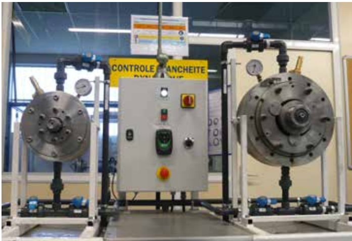
Sealing control test bench
