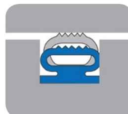
**Figure 3: Low-pressure seal profile**
