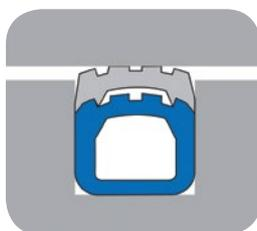
**Figure 2: High-pressure seal profile**
