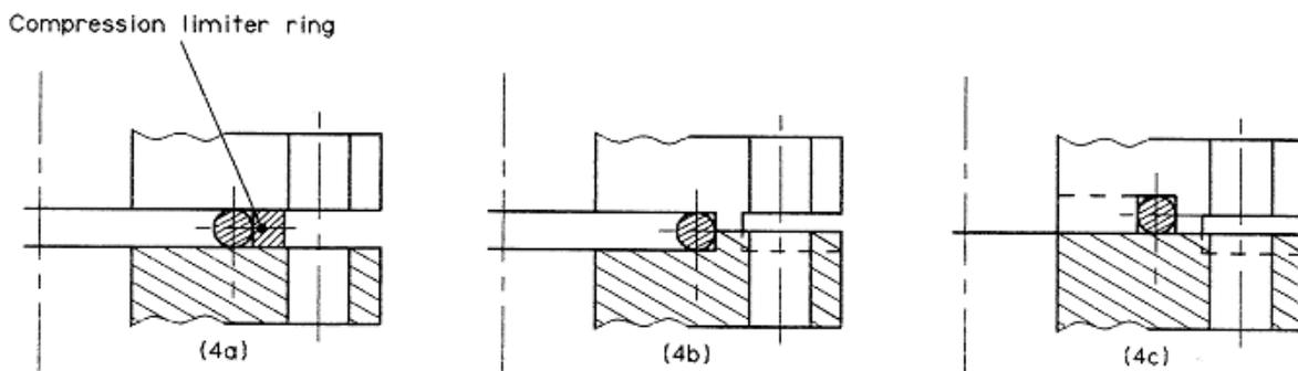
Figure 4. Typical metal-to-metal assemblies
