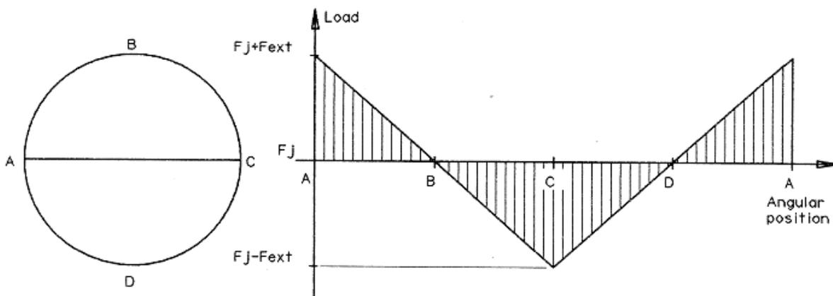
**Figure 3. Load distribution on a non metal-to-metal gasket in bending moment situation**
