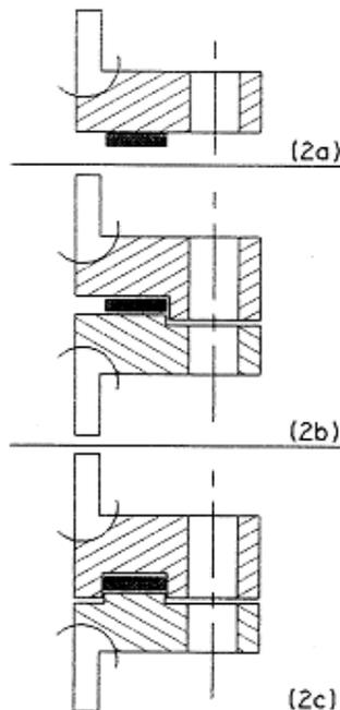
**Figure 2. Standard non metal-to-metal assemblies**
