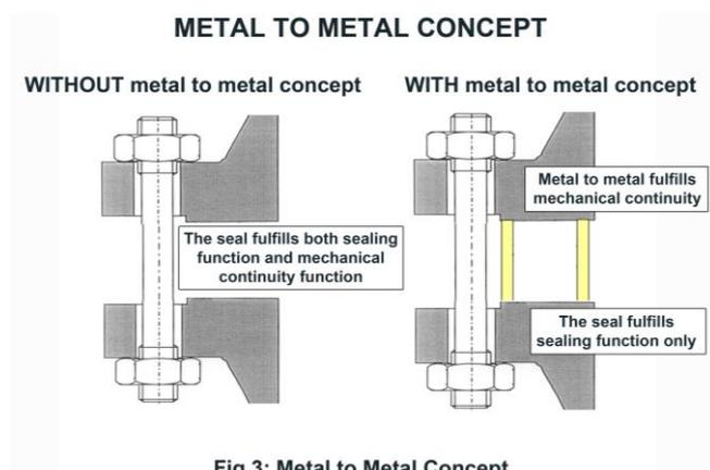
The metal-to-metal concept provides nuclear power plant systems with the ability to seal mechanical joint assemblies together regarding the following criteria:
