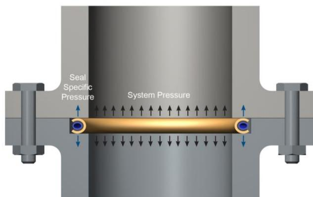
Fig. 2: Typical Bolted Mechanical Joint
