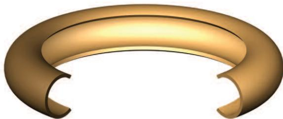
**FIGURE 1. Metal C-ring seals provide greater resilience and require less load than ring joint flange seals but are largely restricted to higher pressure applications. (Source: Technetics Group)**
