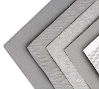
FELTMETAL™ media is an engineered, porous material made by the sintering of metal fibers. Fiber size, porosity and thickness combine to control the desired flow and sound absorption properties. FELTMETAL™ media is produced from fibers having diameters ranging from 50 to 150  $\mu$ . The finer diameter media offers the advantages of lower weight and lower NLF, while the larger diameter media provides enhanced structural strength and better oxidation resistance. The fibers are available in:
