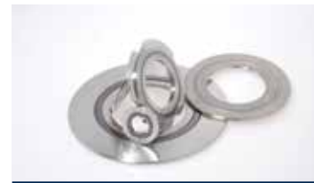
ORIGRAF® GRAPHITE SEALS Unlike flexible graphite cut gaskets, the compression of the ORIGRAF® dieformed seal is limited by a mechanical stop: groove or inner and/or outer ring.
