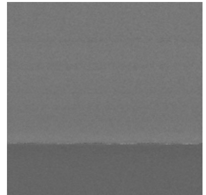
High magnification of the deposited film demonstrates zero voids
