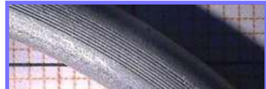
GOOD FLANGE FINISH - CONCENTRIC MARKS
