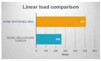
Example with a 3.2 mm torus nickel HELICOFLEX® seal
