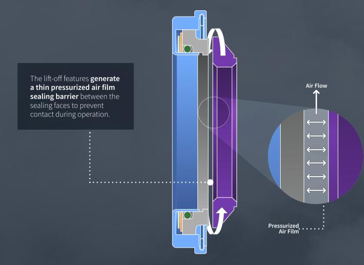
Non-contacting = negligible wear rate, low operating temperature, and longer seal life.
