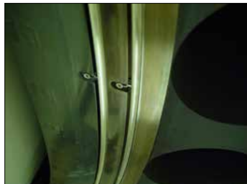
RPV O-FLEX™ Seals with installation clips
